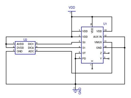
Figure 1: KXPB5 connection to a microcontroller
